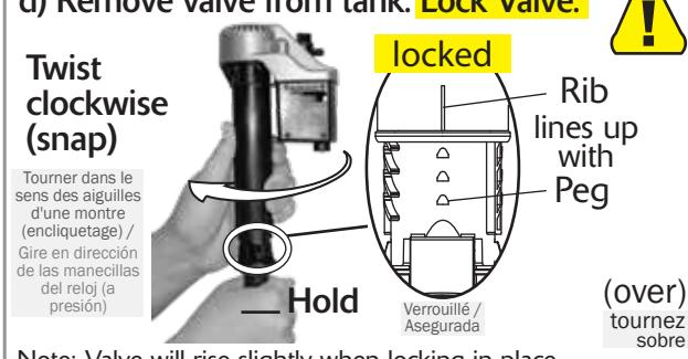
Note: Valve will rise slightly when locking in place.
