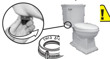
c) Insert metal clip into refill tube.
