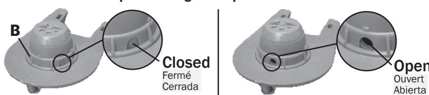
Note: For ease of adjustment, place on flat surface and twist band gently.
