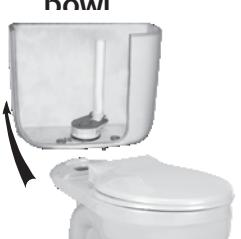
c) Remove sponge gasket. Remove mounting nut (MN), valve, and hardware.
