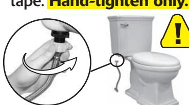
Note: We recommend replacing with a flexible supply line (pictured)
