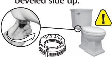
c) Insert metal clip into refill tube.
