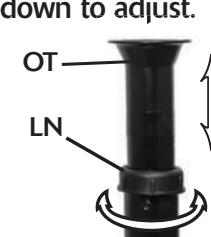
c) Overflow tube (OT) is  $\frac{1}{2}$ " above water line (WL) & at least 1" below flush lever nut (FN). Hand tighten locknut (LN) when done.
