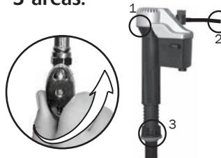
e) Turn off water. Flush. If water level (WL) drops within  $\frac{1}{2}$ " of pencil mark (M), flapper install complete. If not, proceed to next step.
