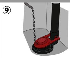
Install toilet flapper with minimal chain slack.
