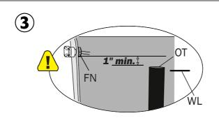
Verify overflow tube (OT) is 1/2" above water line (WL) & at least 1" below flush lever nut (FN). Note: May need to cut overflow tube to proper height.
