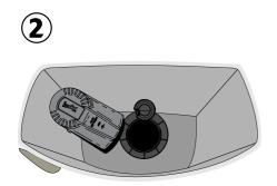
Insert new flush valve into tank opening.
