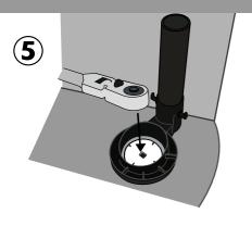
Install 3/8" ratchet into installation tool hole.
