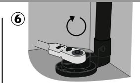
Use downward force on ratchet, begin tightening valve down in clockwise rotation to ensure bottom lip of valve is flush with tank
