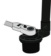
**b.** Rotate counterclockwise rotation to remove flush valve.
